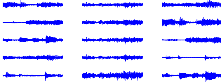
Fig. 7.8. Separation of musical sounds (one second, 10k samples) using Relative Newton method: Left – sources, middle – mixtures, right – separated.
