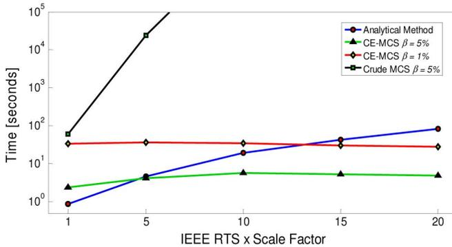
Fig. 6. Performance comparisons—IEEE RTS with different scale factors.
