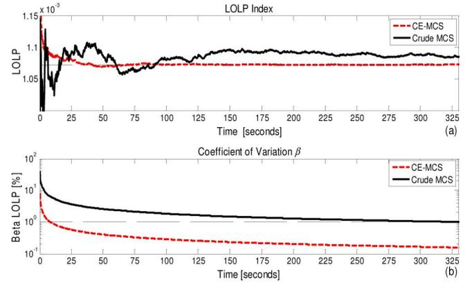
Fig. 4. Convergence process of the LOLP index.
