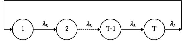
Fig. 2. Multilevel Markov load model.
