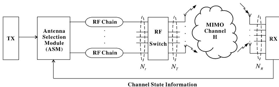
**Fig. 2** MIMO wireless system with antenna selection at the transmitter under CSIT
