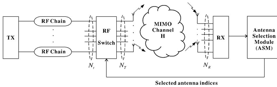
**Fig. 1** MIMO wireless system with antenna selection at the transmitter under CSIR
